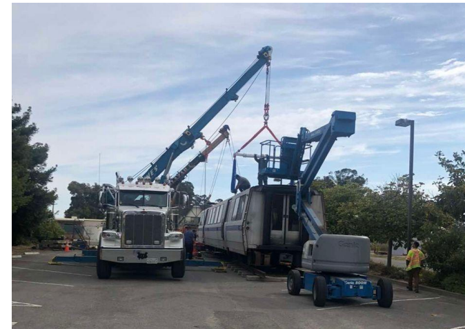
BART train at PEER labs for shaking table testing
