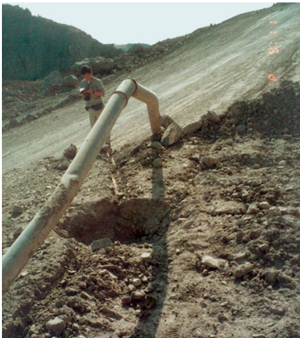
Figure 4.14 – Pipe damaged by reverse faulting in the 1990 Manjil Earthquake in Iran.
