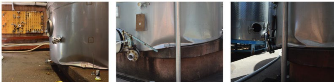
Figure 4.18 – Steel fermentation tank with earthquake-induced damage to tank wall at base.
