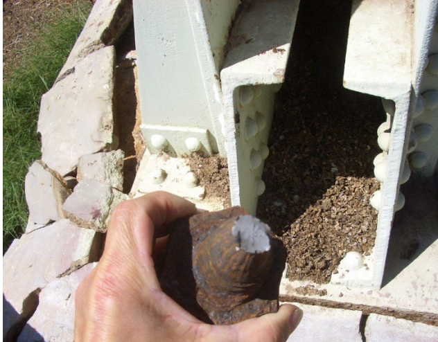
Figure 3.52 – Excessive movement in the structure of the El Centro Water Tower caused rivets to pop. Photo courtesy David Karina.
