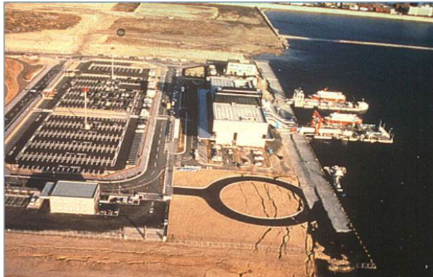
Figure 4.4 – Example of lateral spreading. The earthquake caused the soils to move in the uncontained direction of the body of water nearby.
