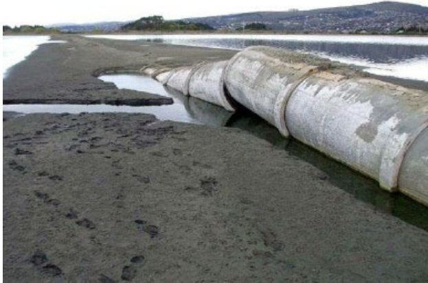
Figure 4.13 – Large asbestos-concrete (AC) pipe damaged by flotation and liquefaction. 2011 Canterbury Earthquake, New Zealand.
