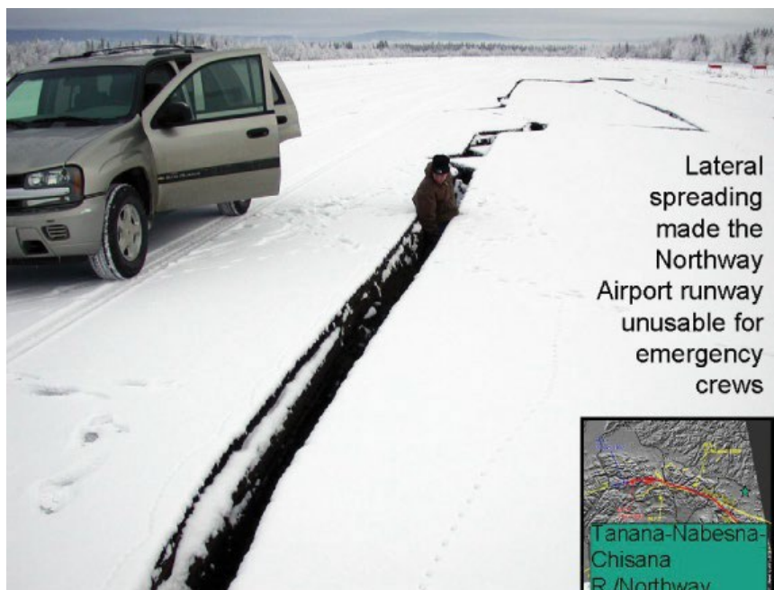
Figure 4.5 – Airport runway in Alaska rendered unusable due to lateral spreading following the 2002 Denali Earthquake. ( Do not step into a developed crevice!)
