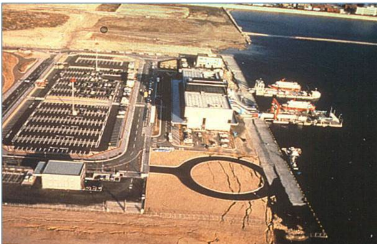
Figure 4.4 – Example of lateral spreading. The earthquake caused the soil to move in the uncontained direction of the body of water nearby.
