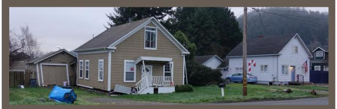
Two homes after the 2022/2023 Ferndale Earthquakes – The house on the left fell off its foundation without retrofitting. The house on the right remained on its foundation due to retrofitting.
