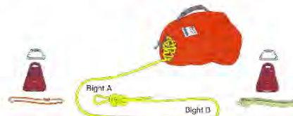
Figure 11-15: How to Construct a 3:1 Pig Rig
