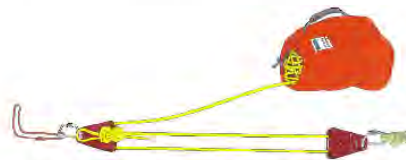
Figure 11-16: Assembled 3:1 Pig Rig
