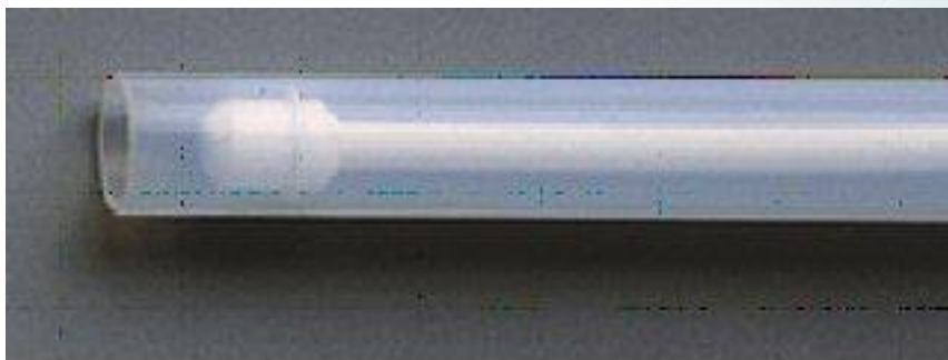
COLIWASA TUBES, 39" to 43" long Teflon, Multi-Use
