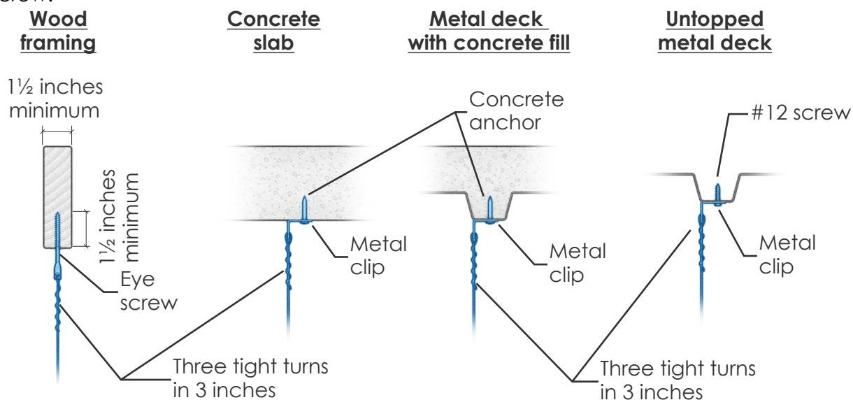
**STEP 3:** Fasten top of 12 gauge ceiling wire by inserting wire through fastener hole and wrapping wire around itself three times in 3 inches.
