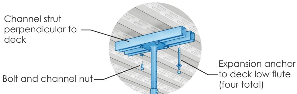
At untopped metal deck: Install channel struts similar to above. Orient the struts perpendicular to the deck direction and space them to match the anchor plate bolt spacing. Attach each channel strut to at least three low deck flutes with two #12 sheet metal screws at each low flute.
