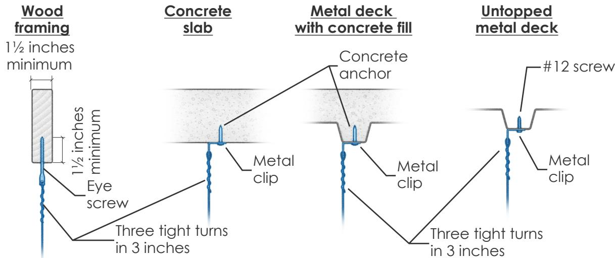
**STEP 4:** Fasten top of 12 gauge ceiling wire by inserting wire through fastener hole and wrapping wire around itself three times in 3 inches.
