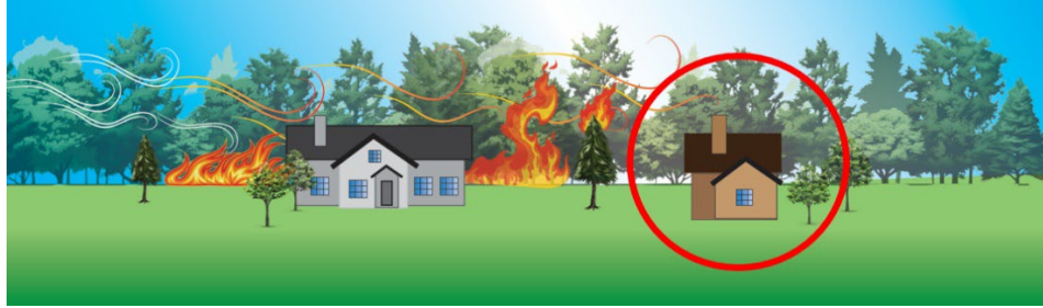
Figure 6. Orient the narrowest portion of the building toward the likely path of wildfire to minimize structure ignition risk (red circle).
