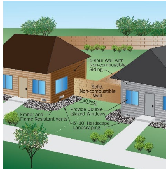
Figure 7. Fire-resistant construction techniques.
