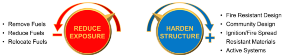
Figure 1. According to NIST's WUI Hazard Mitigation Methodology, WUI fire hazard mitigation is a balance between two input dials--reducing exposure and increasing structure hardening. (Source: NIST HMM)
