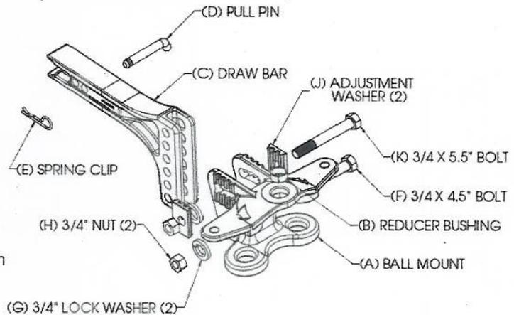
**WARNING: Raised balls usually have reduced load ratings. Ball rating MUST equal or exceed trailer GVWR.**
