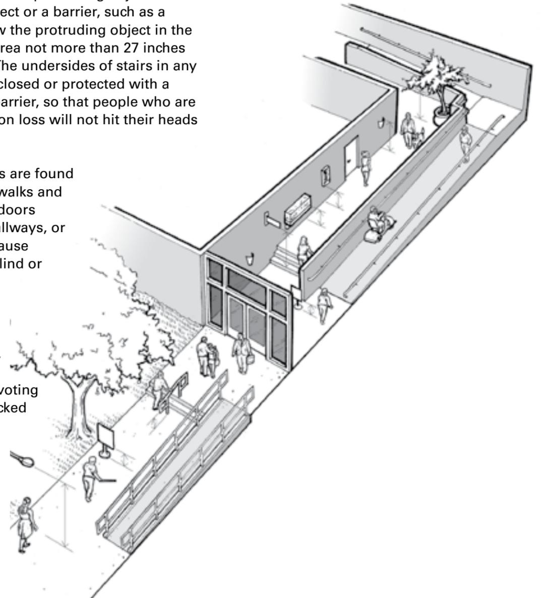
Signs or other objects in the pedestrian route can be a hazard if the bottom is more than 27 inches but less than 80 inches above the route. Objects that overhang the pedestrian route must be at least 80 inches above the route.
