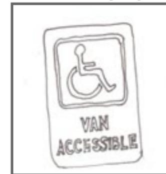
Van accessible parking signs should be used to designate van accessible parking locations.
