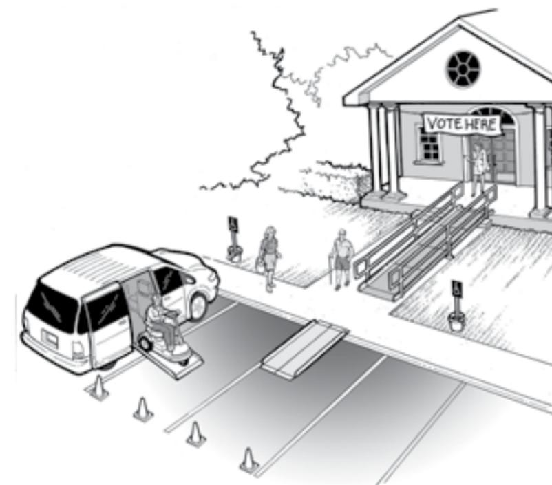
Three standard parking spaces are converted into a van accessible parking space with an access aisle. Cones mark and block off the access aisle and a temporary curb ramp with edge protection connects to an accessible route to the polling place.
