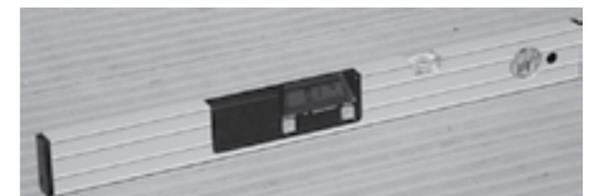
A digital level that can be used with measurements in degrees, percentages, or ratios
