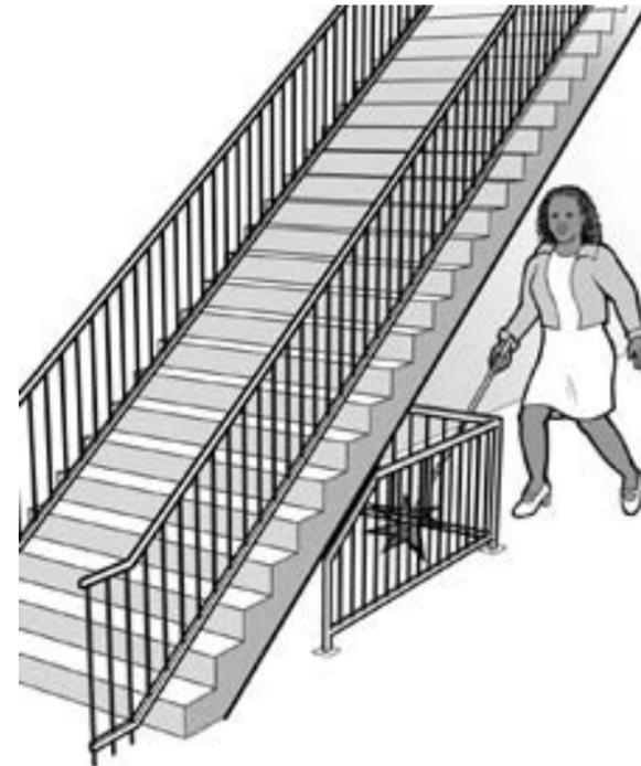
When the underside of a set of stairs is open, it is a hazard to people who are blind or have low vision. Enclosing the area below the stair or installing a cane-detectable barrier helps the person to stop before hitting her head.
