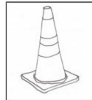
Traffic cones can be used to mark parking spaces, access aisles and passenger loading zones, to hold parking signs, and to warn of protruding objects.
