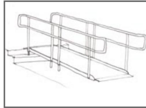
Portable ramps with handrails must be used for heights greater than six inches to provide access over steps. For ramps greater than six inches high, temporary edge protection such as a pipe or piece of wood can be attached with ties or twine to the edges of the ramp. Edge protection must run the entire length of the ramp.
