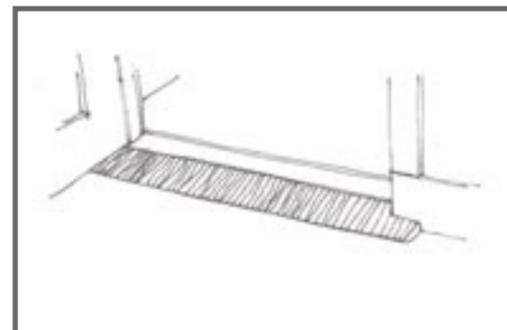
Wedges can provide access at thresholds and slight changes in level.
