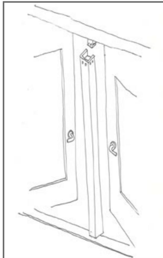
Remove center post between doors if the post is bolted to the door frame to provide a 32 inch clear opening or to allow double doors to be propped open.
