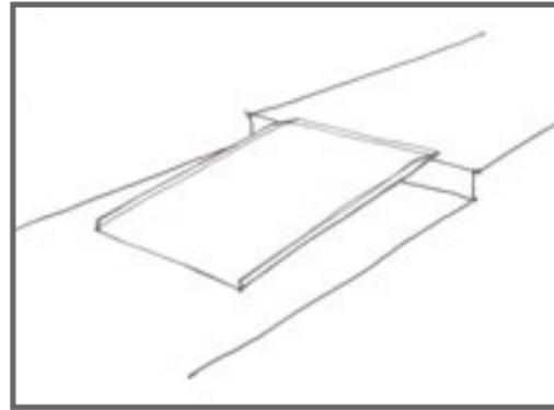
Portable ramps without handrails can only be used for heights six inches or less and can provide access at a curb or low step. Portable ramps also can be placed flat to cover holes or gaps in a sidewalk.
